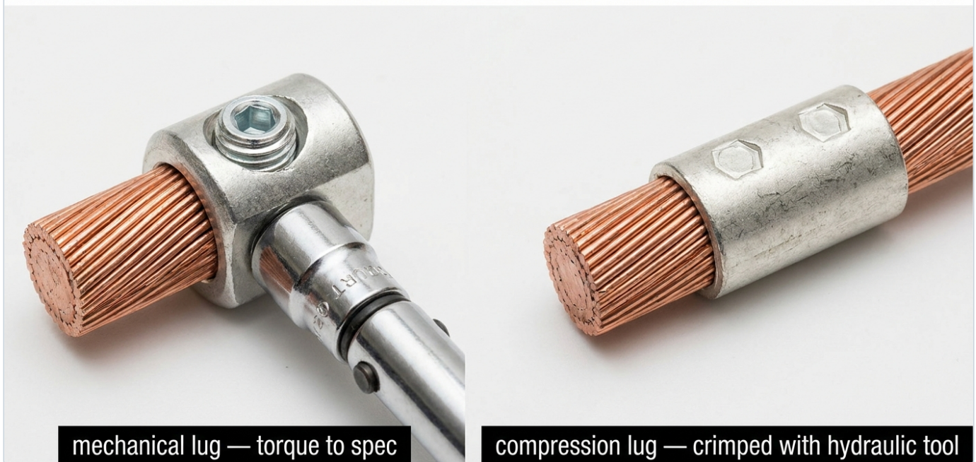
Mechanical set-screw lug (torqued) vs. compression lug (crimped, with die marks).
